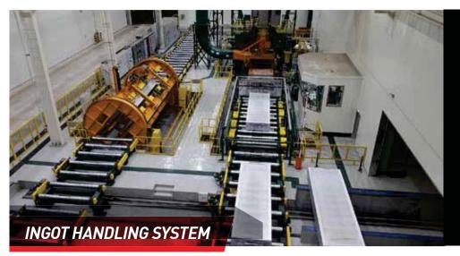
A complete ingot handling system was provided to support a new scalper operation in Asia. Included are roller conveyors, two cross-transfer systems (one is in the depressed floor in the foreground), an ingot turnover device (orange), and an ingot rotator. This equipment was assembled and shop tested in Indiana, then disassembled and packed in shipping containers for ocean transfer. Note the cleanliness of this new facility.
