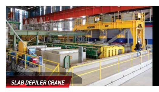
This crane operates in the slab storage area of a hot strip mill in Mexico. Stacks of slabs are delivered to storage saddles, and the crane automatically stages them on the reheat furnace charge conveyor. Magnets are used to grab the slabs, and the hoisting action is hydraulically actuated. Slabs can reach 30' long, and weigh up to 35 metric tons. The semi-gantry style design has a 35' span.
