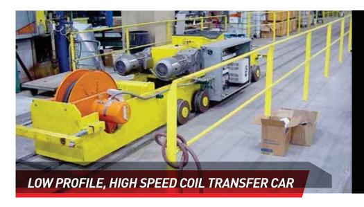
This car and transfer station automates the process of moving coils several hundred feet away from the galvanize line delivery car; a job formerly done manually with an overhead crane. The car is designed to carry coils up to 60" wide, 80" diameter, and 30 tons. It can reach speeds of 235 feet per minute. It is equipped with 8 wheels so that it can smoothly travel over embedded rails crossing its path.
